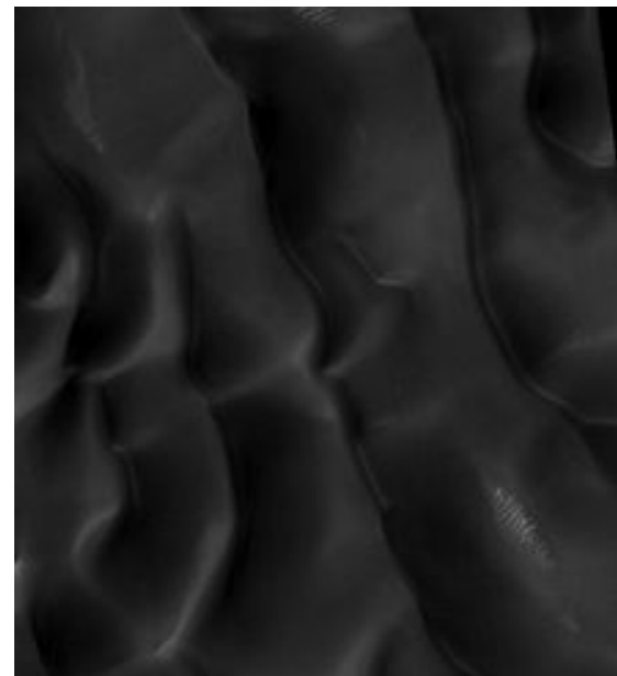
Fig. 3. In the thickest region (no lighter floor can be observed) cassette like surface pattern can be observed on the dark dune layer.
